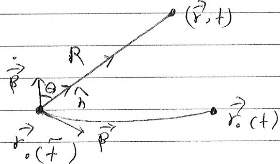
The expressions for  $\vec{E}_{\text{vel}}$  and  $\vec{E}_{\text{rad}}$  are calculated at the retarded time  $\tilde{T}$ , which is the solution to the following equation:
